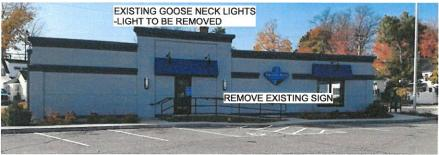
**EXISTING** 70'-0" BUILDING 12'-3 3/4" SIGN BAND PLATE LOGO SIGN C SIGN B NON-ILLUM. FABRICATED CHANNEL LETTERS EQ 3'-0" SIGN 2'-6"± BAND V.I.F. EQ 5' - 5" 6'-0" **NEW GOOSE NECK LIGHTS PROPOSED** (LIGHTS SHOWN AN APPROXIMATION) **INSTALLED BY GC** -TWO ON EITHER SIDE OF SIGN
