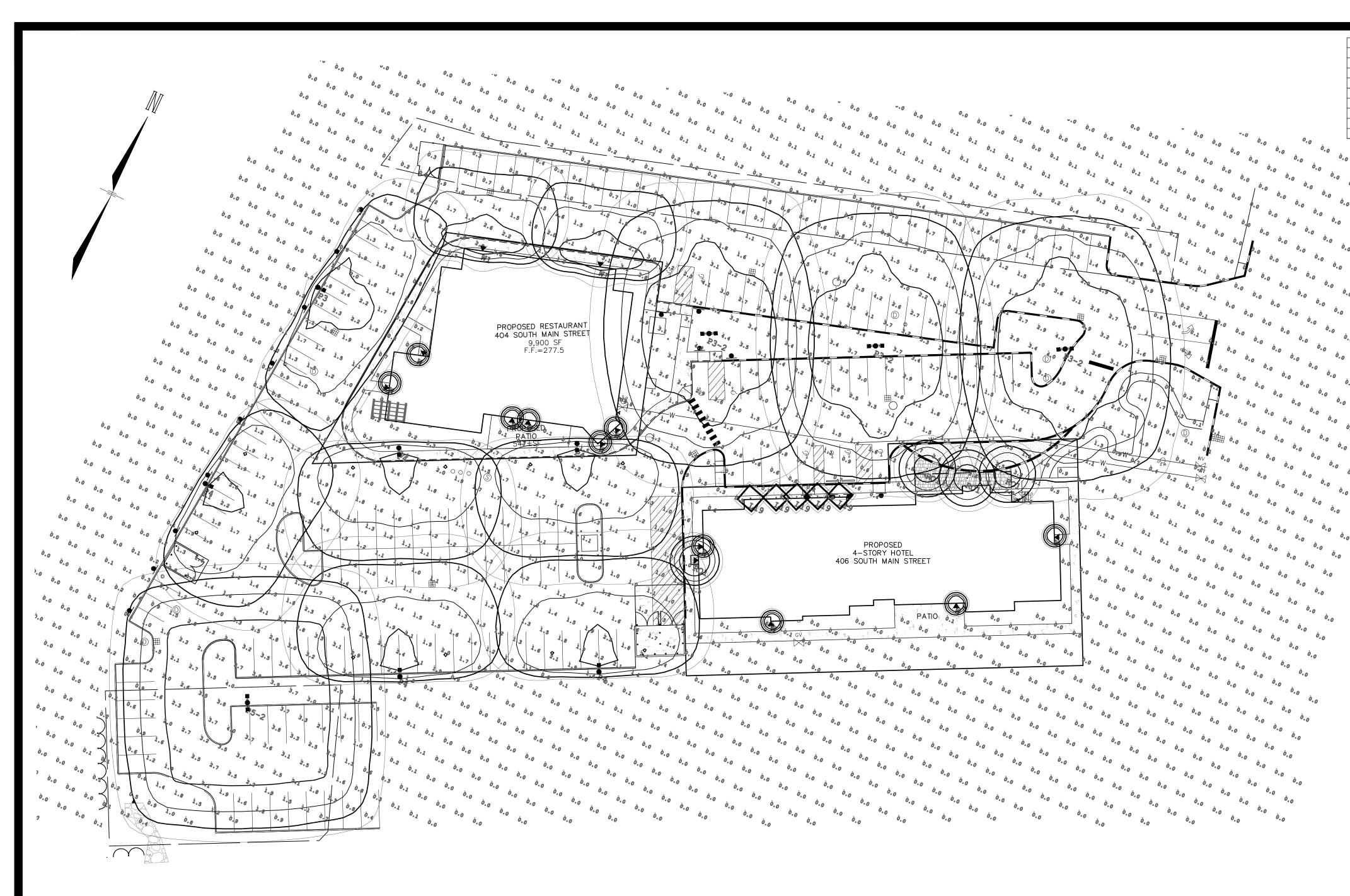
GLEON-AF-02-LED-E1-SL3-800-HSS/SSS4A20SFN1 MTD. ON 3' PEDESTAL BY OTHERS 2-GLEON-AF-02-LED-E1-T3/SSS4A20SFN2 MTD. ON 3' PEDESTAL BY OTHERS GLEON-AF-02-LED-E1-SL4-800-HSS/SSS4A2OSFN1 MTD. ON 3' PEDESTAL BY OTHERS 2-GLEON-AF-03-LED-E1-5MQ-800/SSS4A20SFN2 MTD. ON 3' PEDESTAL BY OTHERS (23' AFG NLCBC65130WW ASPENTI 5 WALL GWC-AF-01-LED-E1-SL4-800/ WALL MTD 15' AFG
