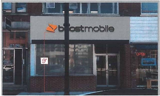
Scope of work; remove existing signage, paint wall facade and patch holes, and install (1) new internally illuminated face lit and halo LED style channel letter set over main entrance. Sign UL listed and tested.
