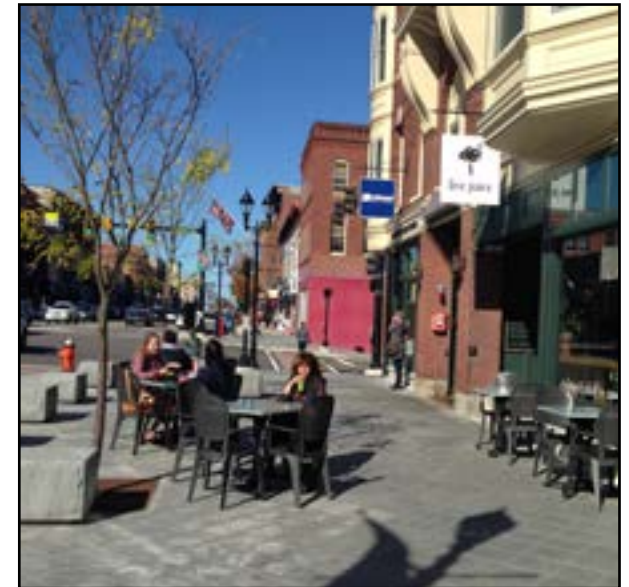
Although Zones are not clearly delineated with paving patterns, dining areas are arranged to avoid encroaching on the pedestrian clear zone or public seating areas.
