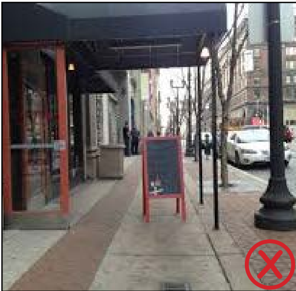
Sign is placed in the middle of the pedestrian clear zone, blocking free movement and creating an uncomfortable pedestrian space.
