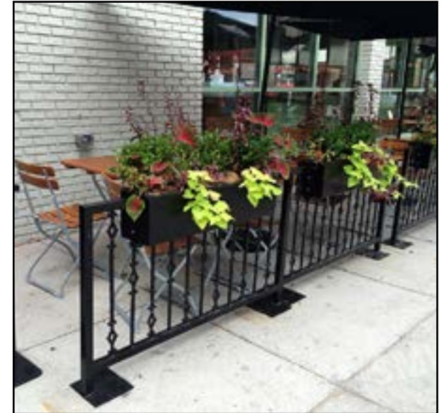
Outdoor dining enclosure utilizes quality materials, creates a sense of privacy with planters, has substantial base plates for stability, and takes up minimal space.
