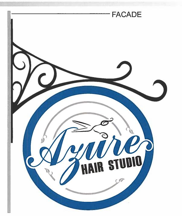
DOUBLE SIDED, 36" ROUND, COMPOSITE MATERIAL SIGN, MOUNTED ONTO FABRICATED DECOR SCROLL BRACKET.
