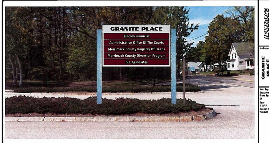
Overall sign dimensions are 5' tall x 8' wide, granite posts with aluminum directory panels with vinyl copy header panel has raised letters. Ground to top of sign is 9' 6" Zone IS allows 40 sqft freestanding sign
