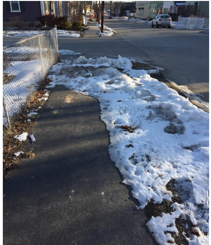
Figure 4: In this photo, snow removed from a storm drain was piled onto the sidewalk in early winter, leaving an icy blockage not easily removed by sidewalk plows. A condition like this can persist through the remainder of the winter.
