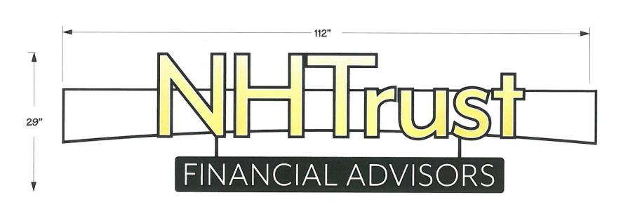
112" X 29" dimensional sign with two layer prismatic carved HDU letters finished with 23k gold leaf, black backer letters, solid steel frame made from 1/2" sq. rod, lower panel to be raised acrylic letters and black smalt background, details to match front sign. \$5340 Installation.
