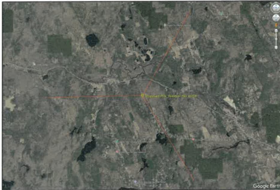
Figure 2b: Typical Sector Azimuths for PWS Facilities (Alpha 30°, Beta 150°, and Gamma 270°) Near Map 2 Lot 8, 2nd NH Turnpike, Windsor, NH (Picture courtesy Google Earth ©2026 and may not represent current conditions)
