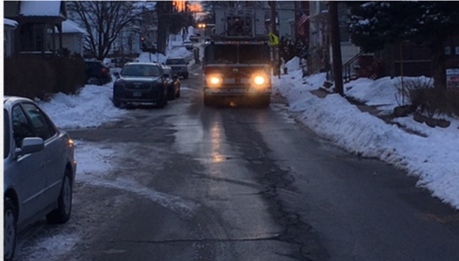
Warren Street (Green to Rumford) 26-27.7 +/- Wide; 2-Way Traffic (Parking South Side Only) 15 Parking Spaces 70% Average Utilization (Weekday 8AM – 6PM) Potential Recommendation: Eliminate On-Street Parking 45
