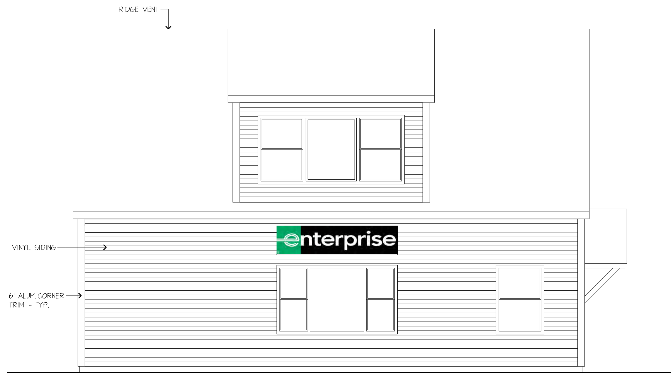
2 EXISTING NORTH ELEVATION SCALE: 1/4" = 1'-0"
