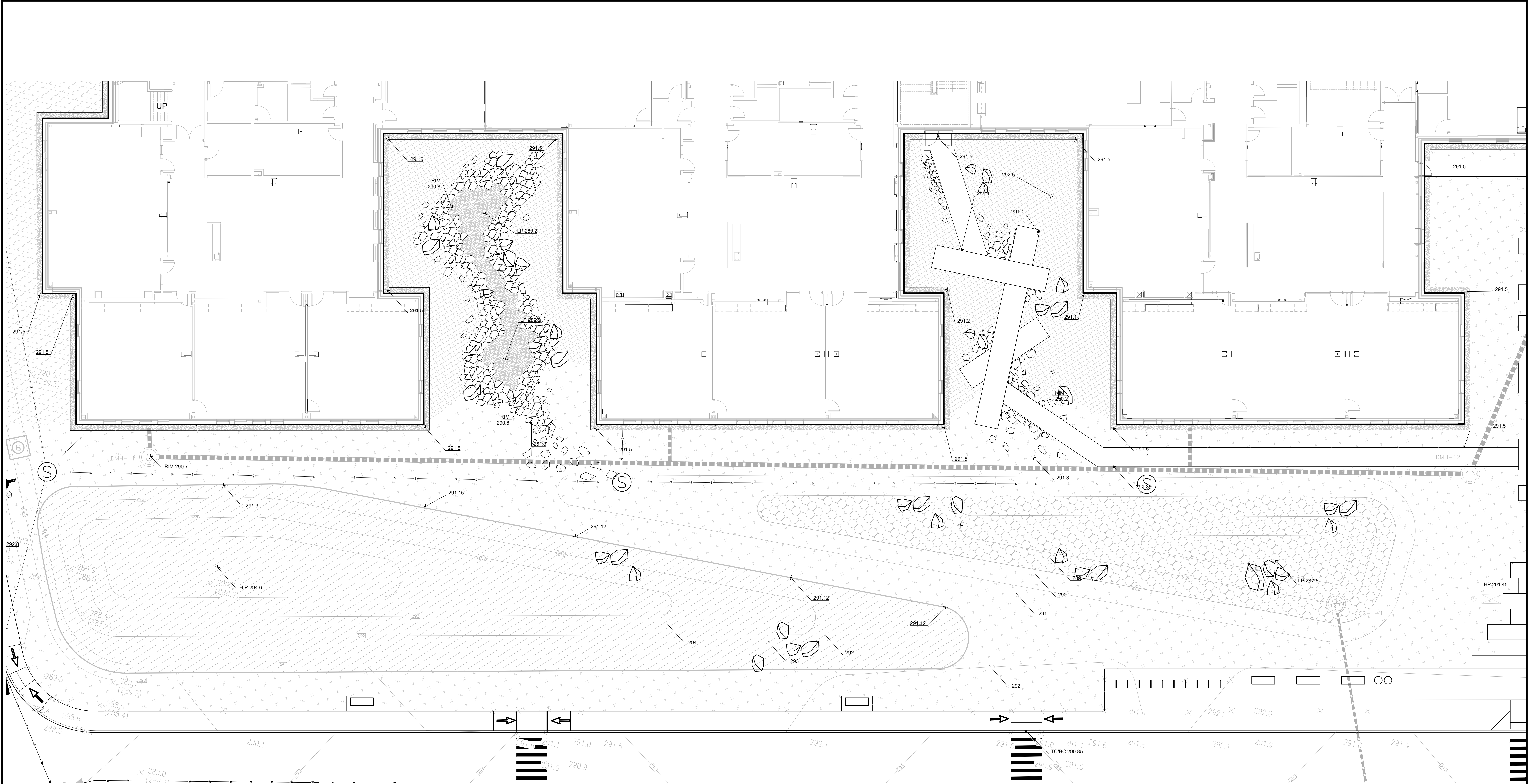
1 SOUTHERN COURTYARD ENLARGEMENT - GRADING PLAN SCALE: 1"=10'-0"
