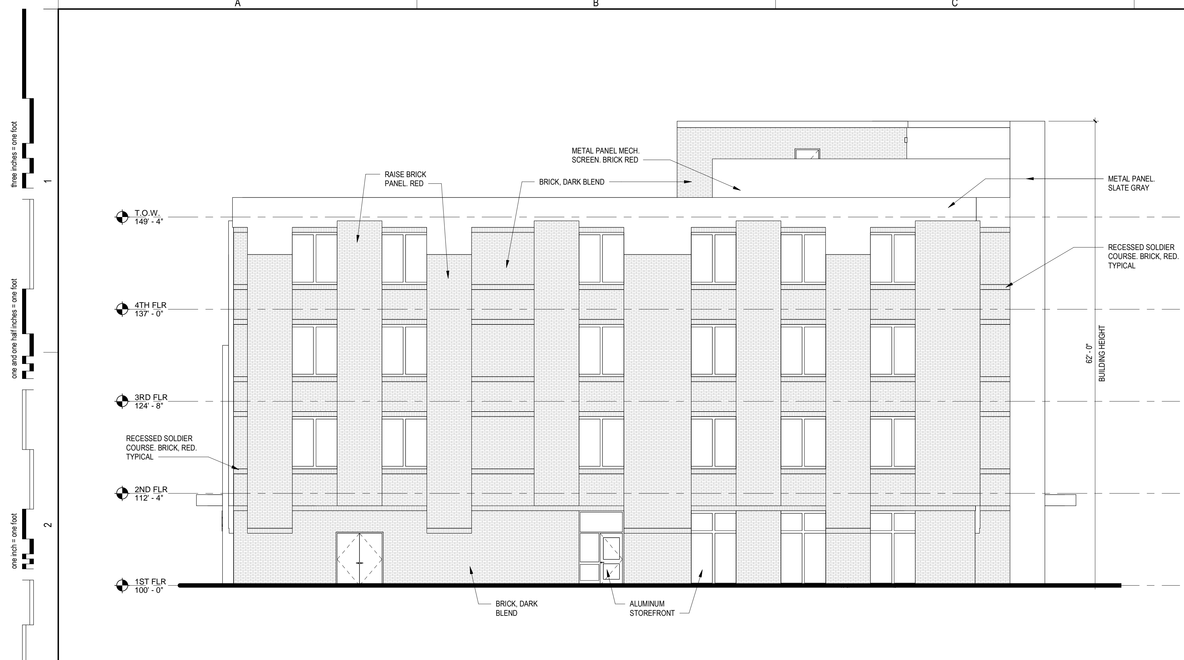
1 EAST BUILDING - LEFT ELEVATION 1/8" = 1'-0"
