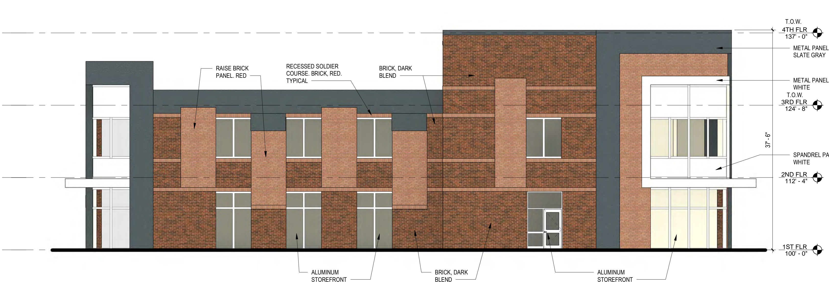
WEST BUILDING - LEFT ELEVATION
