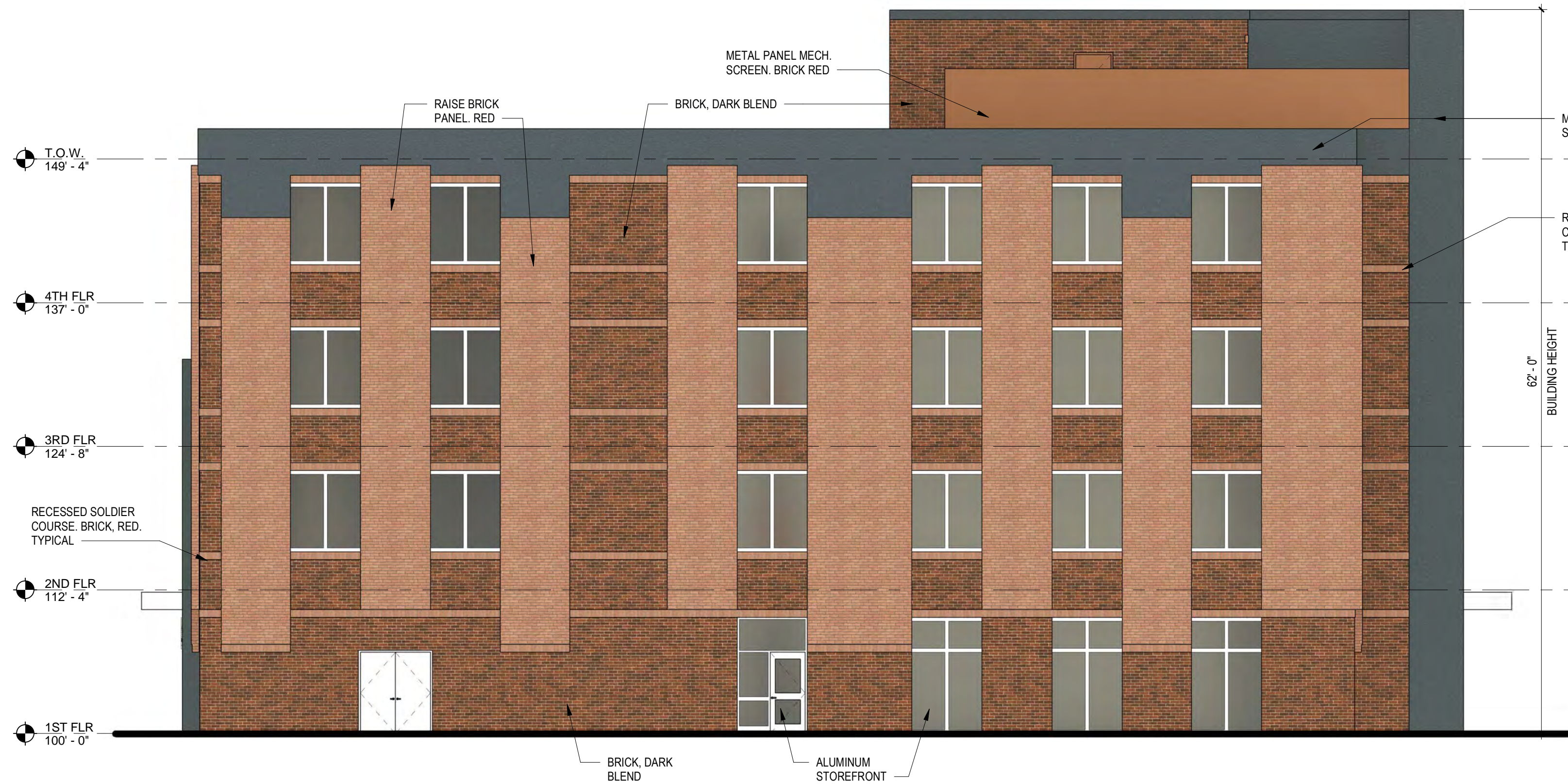
EAST BUILDING - LEFT ELEVATION
