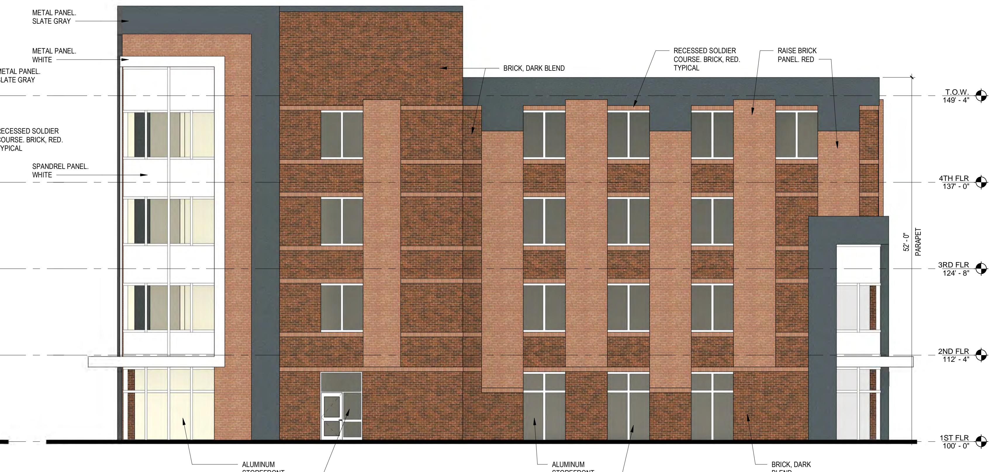
EAST BUILDING - RIGHT ELEVATION
