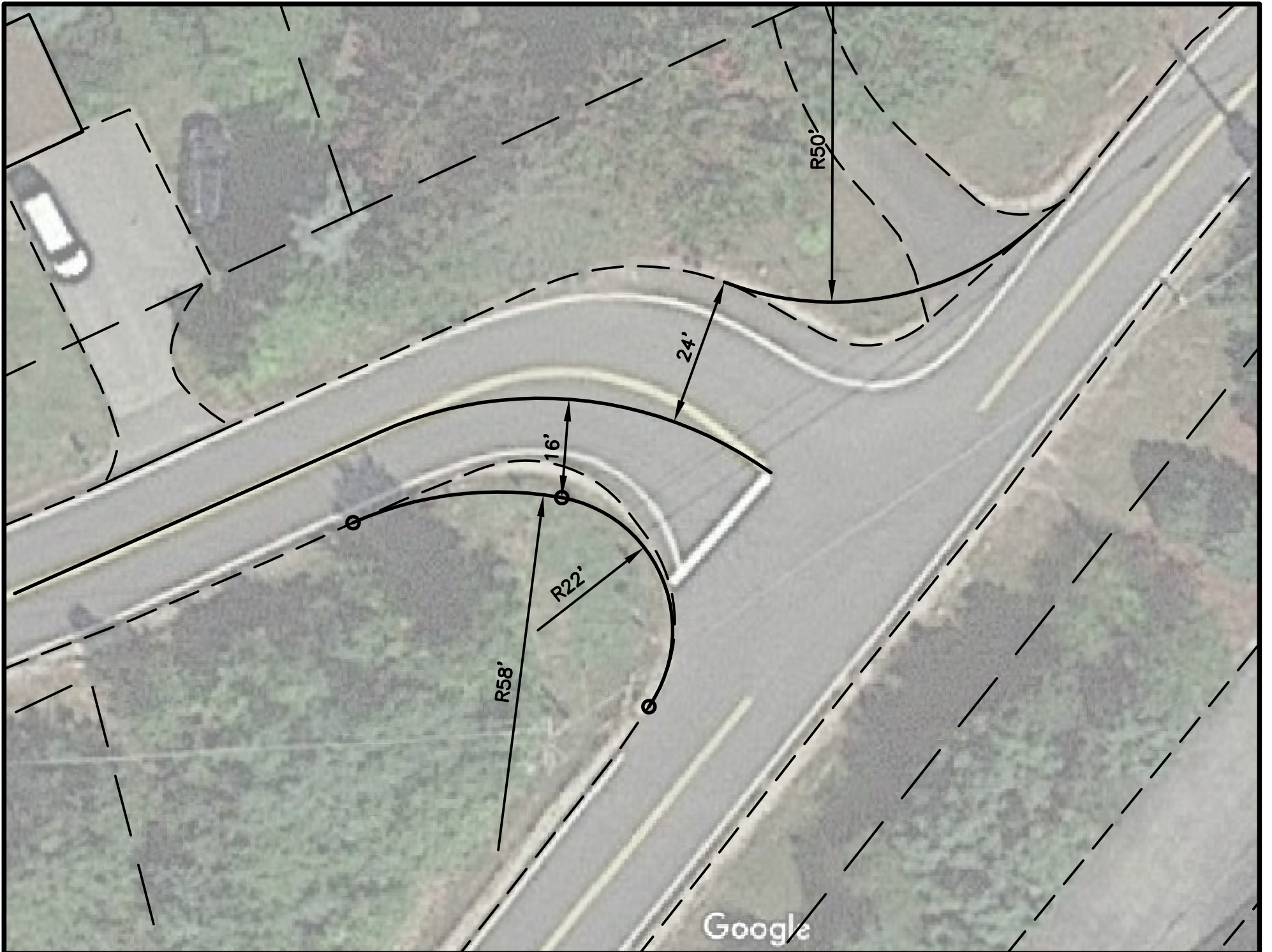
Alternative C - Widen 2 Sides, Eastward Skew
