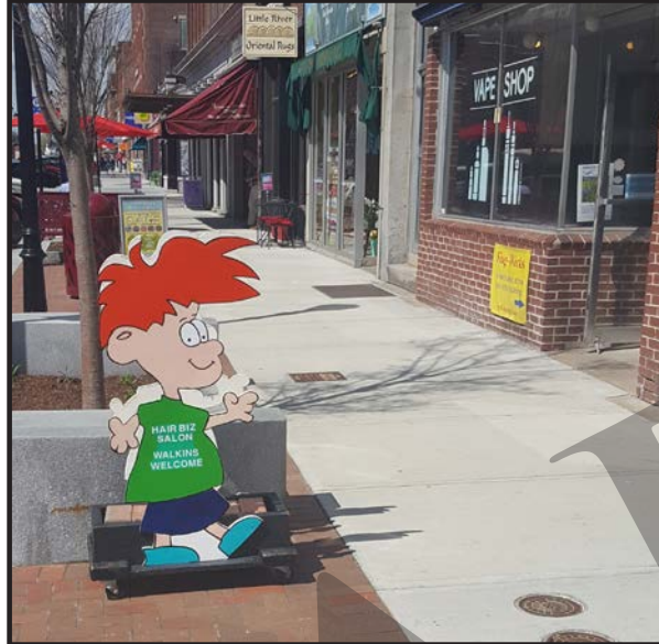
Playful and colorful sign is located correctly, out of the pedestrian clear path
