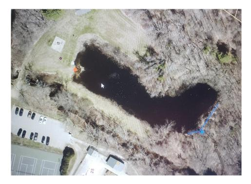
The red dot on the left side of the pond is the inlet, the blue dot on right is outlet while the blue line shows the location of the small earth dam.
